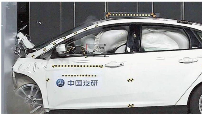
Fig. I.4 Measurement of Distance between Center of Steering Wheel and Front End of Side Head Protection Airbag
