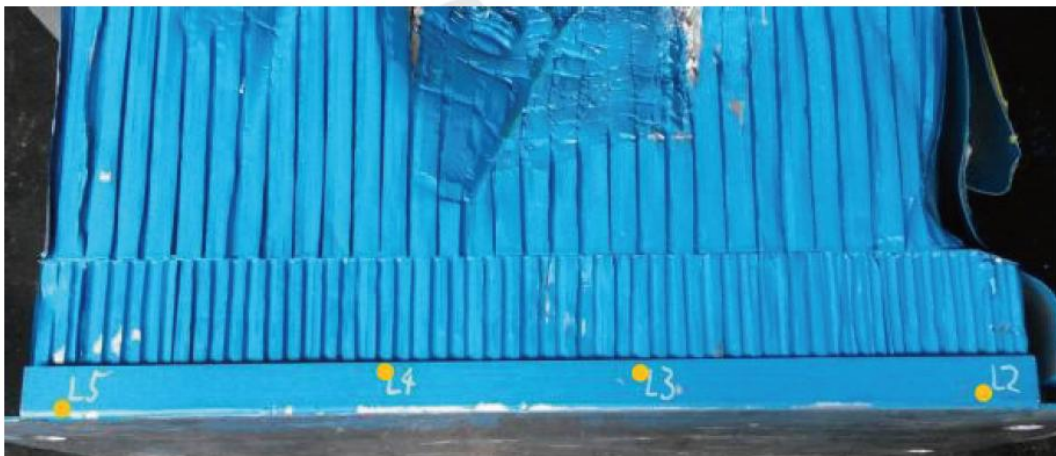
Fig. C.8 Schematic Diagram of Reference Point for Barrier Deformation Measurement
