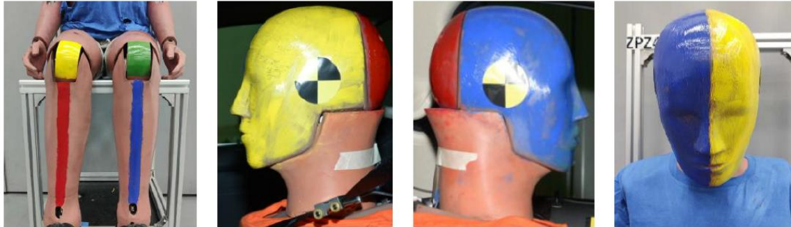
Fig. B.3 Schematic Diagram of ATD Painting
