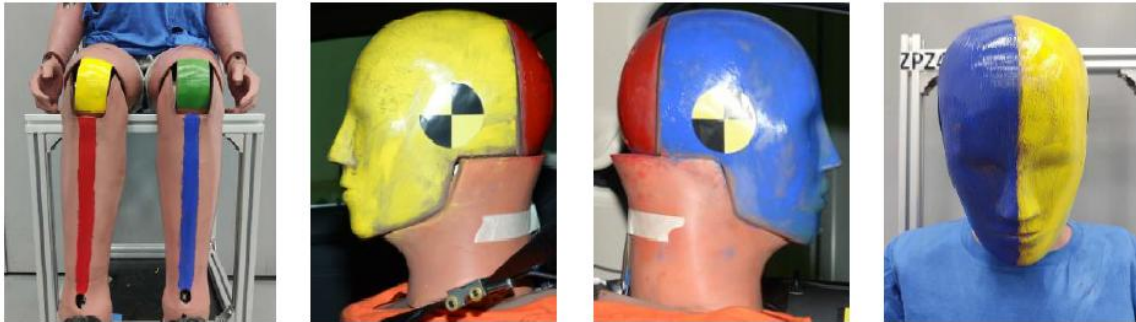
Fig. A.3 Schematic Diagram of ATD Painting
