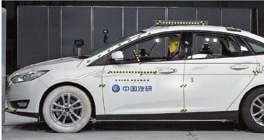
Fig. I.1 Measurement of Distance between Lock Catch Mark of Rear Door and Center Mark of Steering Wheel
