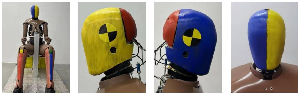
Fig. C.1 Schematic Diagram of ATD Painting (THOR 50 th ATD)
